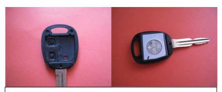
Once your silicone buttons are fitted in, place electronic board back in remote, cover it with bottom part of the shell and screw it together. **No reprogramming is need it** as remote will work straight away.
