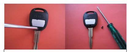
Unscrew holding screw located at the back of your remote key.
