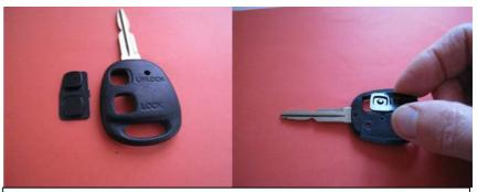
Silicone buttons will be fitted from inside of the remote. Simply press fit silicone buttons in.
